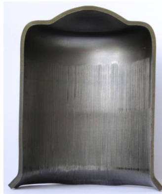
Figure 6 – Condition of the outer and inner surfaces of the semi-finished product after the first calibration.
