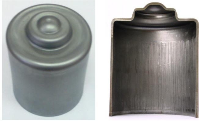
Figure 10 – Condition of the outer and inner surfaces of the semi-finished product after height calibration.
