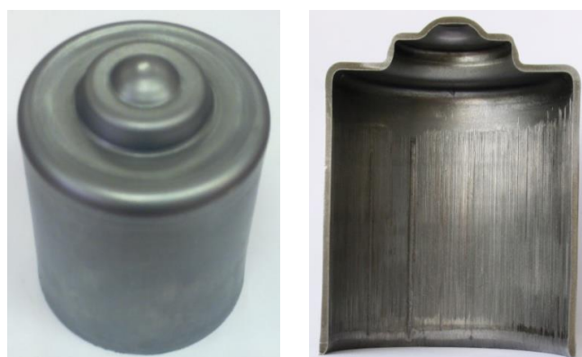
Figure 9 – Condition of the outer and inner surfaces of the semi-finished product after cutting of flange.
