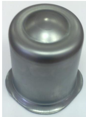
Figure 6 – Condition of the outer and inner surfaces of the semi-finished product after the first calibration.
