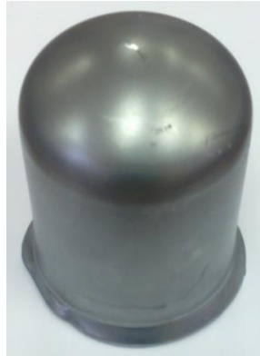
Figure 5 – Condition of the outer and inner surfaces of the semi-finished product after the third drawing.
