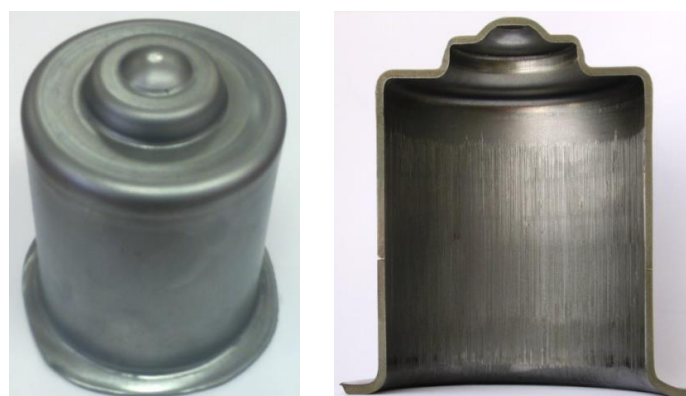
Figure 8 – Condition of the outer and inner surfaces of the semi-finished product after the third calibration.
