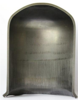
Figure 5 – Condition of the outer and inner surfaces of the semi-finished product after the third drawing.
