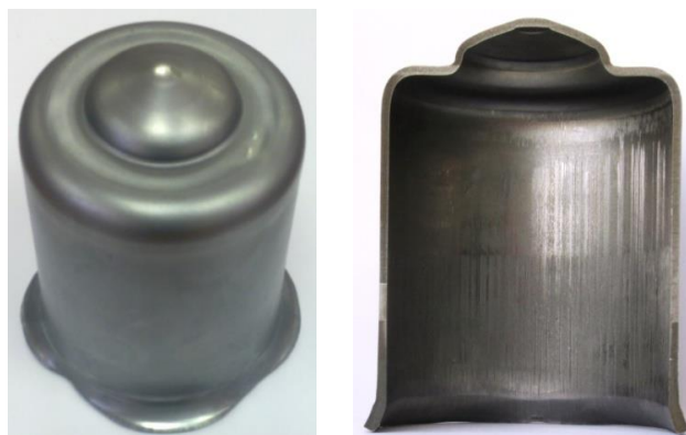
Figure 7 – Condition of the outer and inner surfaces of the semi-finished product after the second calibration.
