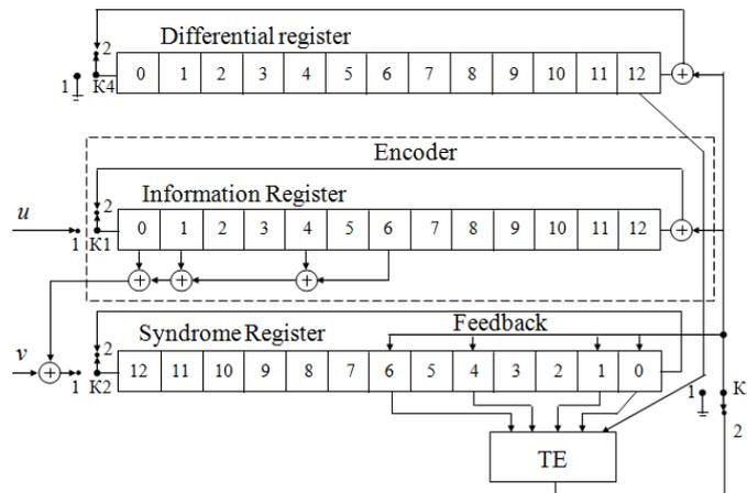
**Figure 5. High-precision iterative decoder HICC with  $r=1/2$ ,  $d=5$ ,  $n=26$  and  $g(x)=1+x+x^4+x^6$ . The upper inputs of the cells 0, 1, 4 and 6 of the register of the syndrome are assumed to be inverting**
