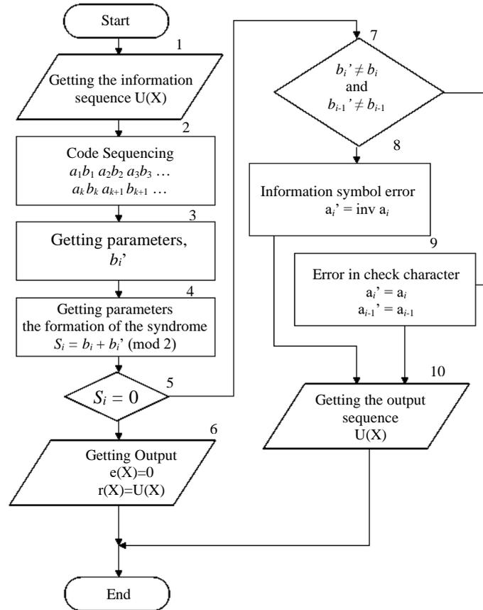
Figure 8. HICC decoding algorithm (APP Decoder 1)
