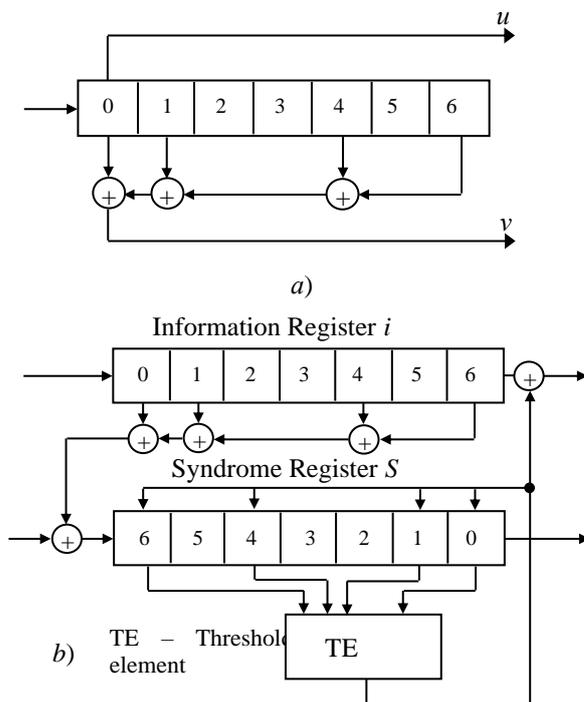
Figure 3. Scheme of error-correcting encoder (a) and TD (b) convolutional self-orthogonal code
