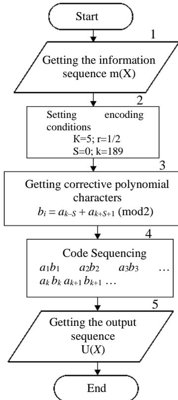
Figure 6. Encoder Algorithm HICC
