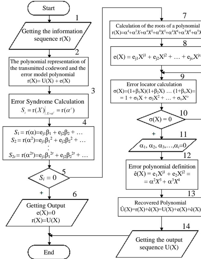
Figure 9. HIBC decoding algorithm (APP Decoder 2)
