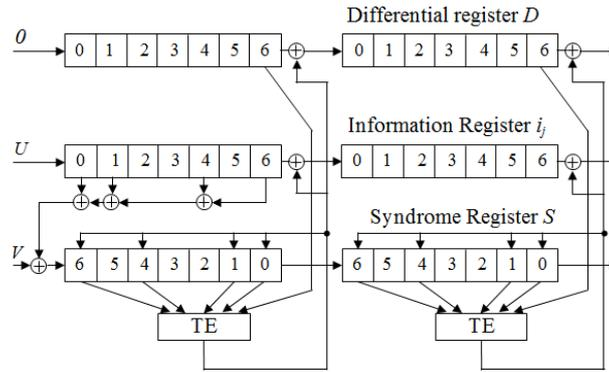
**Figure 4. Structural diagram of the MTD convolutional SOC with  $r=1/2$ ,  $d=5$  and  $n_A=13$  for two iterations of decoding**
