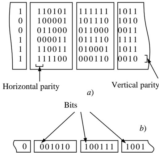
**Figure 1. Parity check for serial (a) and parallel (b) the structure of the iterative code**
