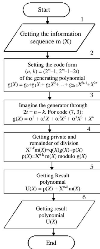
Figure 7. Encoder Algorithm HIBC
