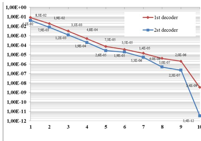
FIGURE 11. ERROR PROBABILITY  $P_b$  IN BITS OF THE NUMBER OF ITERATIONS ( $E_s/N_0 = -1,32$  DB,  $E_B/N_0 = 1,70$  DB)
