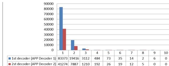
FIGURE 12. THE NUMBER OF ERRORS IN BITS OF THE NUMBER OF ITERATIONS ( $E_s/N_0 = -1,32$  DB,  $E_B/N_0 = 1,70$  DB)
