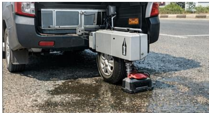
Figure 6. Pavement skid resistance testing.
