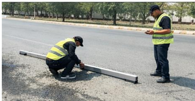
Figure 1. Road roughness measurement using straightedge device.
