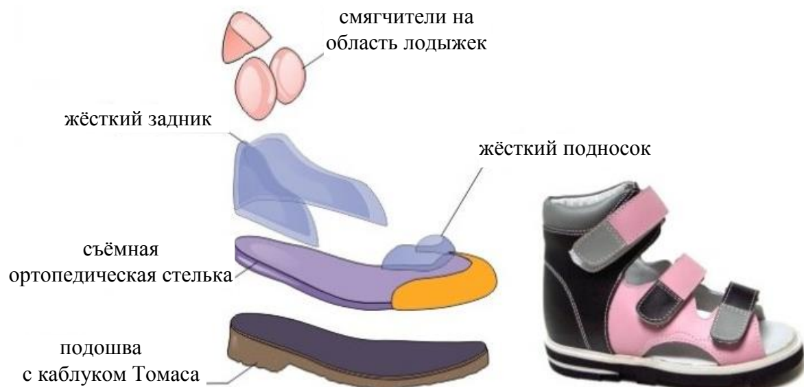
Figure 29. Characteristics of corrective parts of shoes for children with varus and valgus foot deformities
