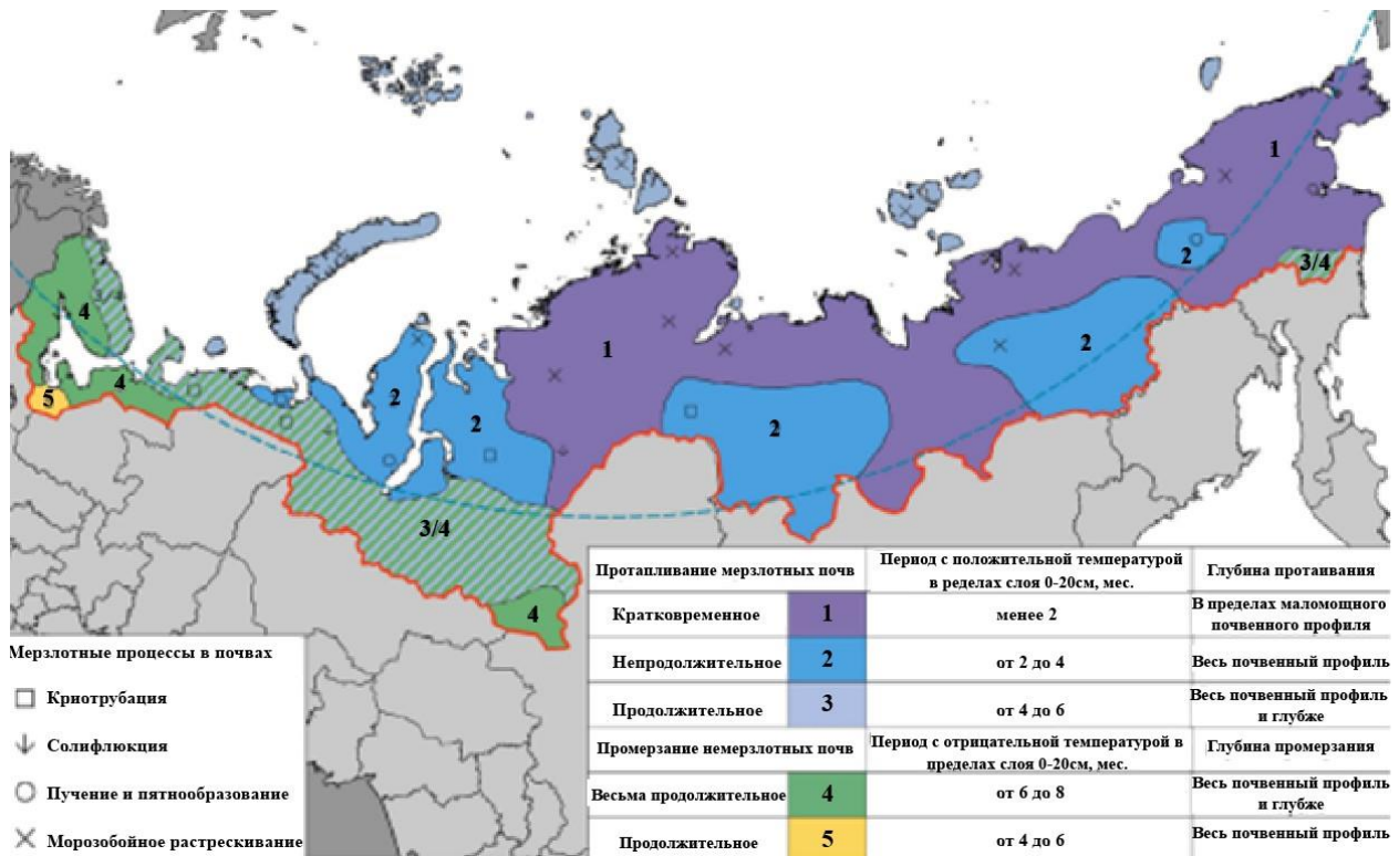
Figure 10. Map of permafrost processes in the Arctic zone of the Russian Federation
